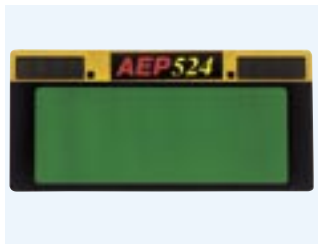
AEP524 Lens Part No. AEP524-0 Shade 11 auto-darkening lens, fits most standard helmets and can be used to upgrade the WGAC10 helmet. Lens area 52mm x 108mm.
