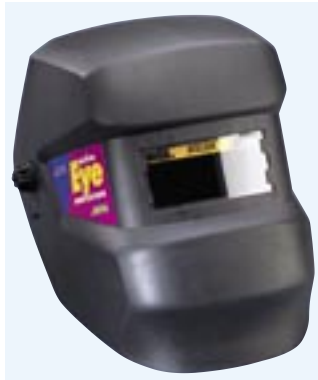
AEP11 Helmet Part No. AEP11-0 Basic lens auto-darkens to shade 11 when arc is struck. Can be upgraded to shade 12.5 by using a shade-on lens. Lens area 52mm x 108mm.
